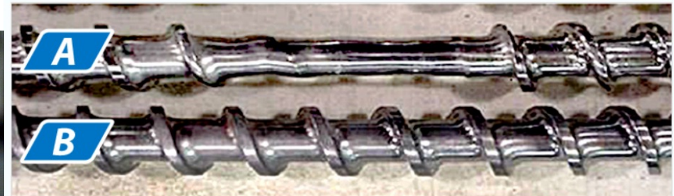
A : Abrasive wear resistant screw after 6 month processing highly abrasive ceramic filled polymer B : Tungsten carbide coated screw after 12 month in the same process
