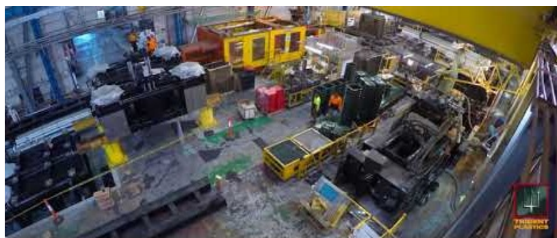
ENGEL duo 5500 with a clamping force of 55,000 kN
