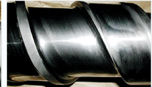
105mm screw after 10 months processing Nylon+GF40%
