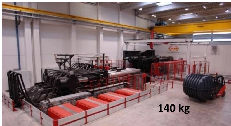
ENGEL duo 5500 with a clamping force of 55,000 kN
