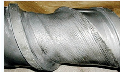
105mm screw after 3 months processing Nylon+GF40%
